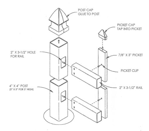
in the picket. You may need to rock the clip back and forth to lock it in place. Make certain to insert the thick end into the picket. Place the picket down over the rails and, with the palm of your hand, firmly seat the clips. When complete, stand the
