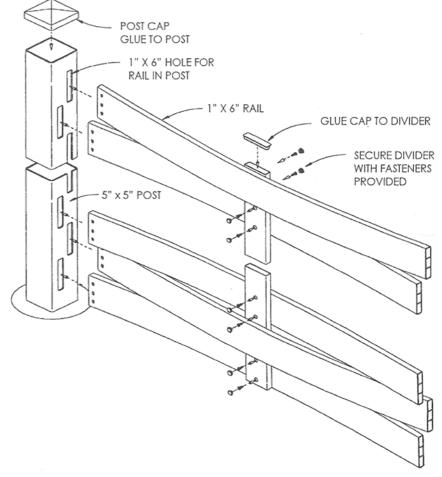
vider using the fasteners provided. (Note: fasteners may differ from photo)
